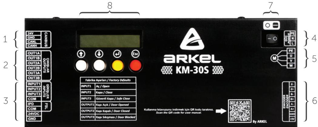
• Door Controller Internal Structure
